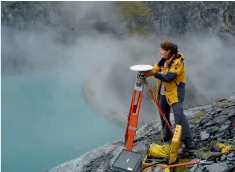
High-precision GPS observations in the three-dimensional control network for the pump storage plant 'Linthal2015' (Canton Glarus).
