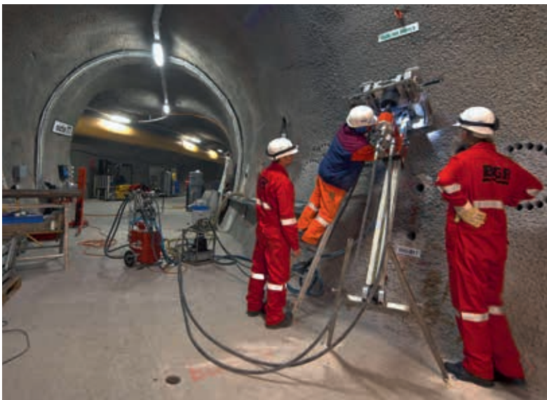
Researchers from the Federal Institute for Geosciences and Natural Resources in Hannover, Germany (Bundesanstalt für Geowissenschaften und Rohstoffe BGR), make a boring in the Rock Laboratory Mont Terri (Canton Jura) to extract opaline clay cores.
