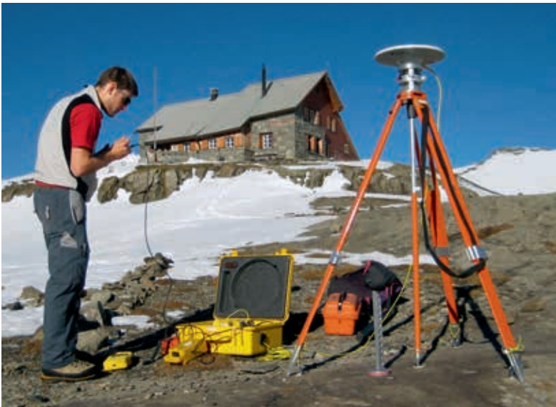
GPS observations in front of the Muttsee hut (Canton Glarus). Nation-wide, high-precision GPS surveys can be carried out thanks to the new national surveying network LV95, the permanently operated reference stations of the Automated GPS Network of Switzerland (AGNES) and the positioning service swisstopo established and operated by swisstopo.
